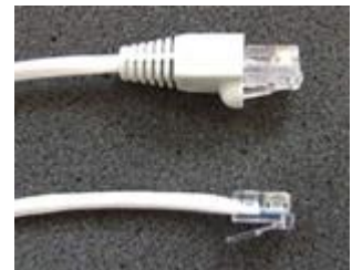
Top cable is an Ethernet cable, the bottom cable is a standard phone line cable.
